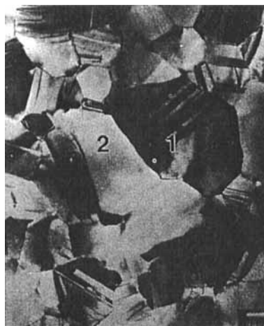
Typical microstructure of the \alpha_1 + \text{AuCu}_3 samples.
