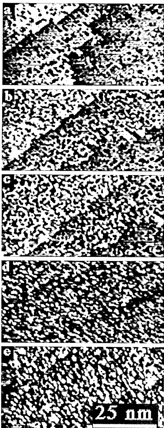
Fig. 10. Si growth from \text{Si}_2\text{H}_6 at T=620 K and P=6 \times 10^{-7} Pa (filled-states image).
