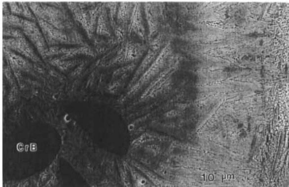
Typical secondary-electron SEM image of the AISI 1045 steel laser alloyed with CrB.
